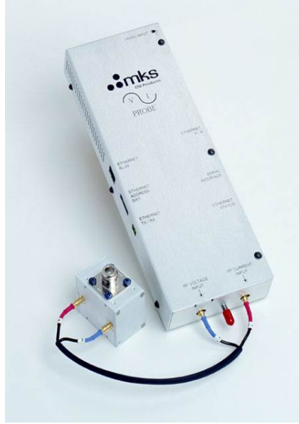
Figure 2.9: Photo of entire MKS VI probe system[2].
