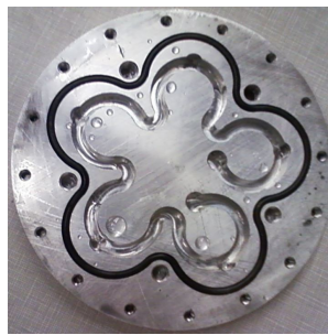
Figure 2.6: The center shows the flower patterned water channel surrounded by an O-ring and the holes for the bolts to hold it all together.
