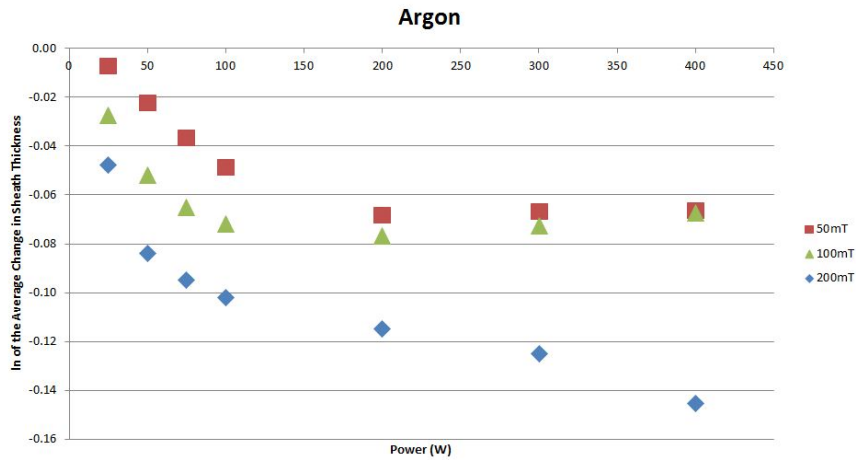
Figure 3.10: Region D for an argon plasma in a power sweep of the 28.476 MHz pulsed generator.
